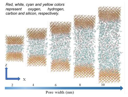
Snapshot of the simulation cells containing silica surfaces with  $CO_2$ , toluene and propane molecules in confinement.
