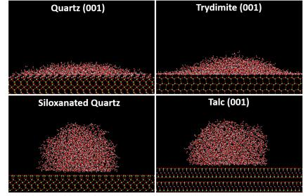
MD simulation results for water sessile drops (7nm diameter) at selected silica surfaces after 1ns. Color codes for atoms: green, N; lime, Si; blue, Mg; red, O; white, H.
